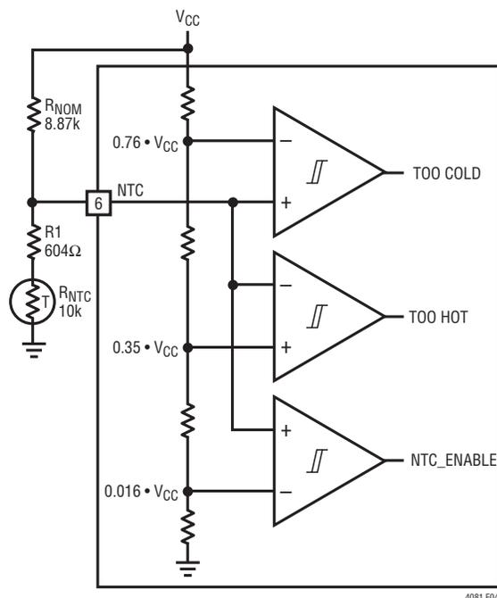
Figure 4. NTC Circuits
