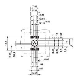
Soldering pad geometry
