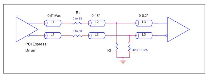
Figure 11B. Recommended Termination (where a point-to-point connection can be used)
