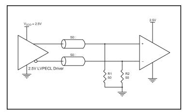
Figure 10B. 2.5V LVPECL Driver Termination Example
