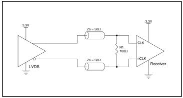
Figure 7E. CLKx/nCLKx Input Driven by a 3.3V LVDS Driver
