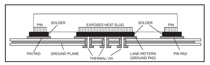
Figure 13. P.C. Assembly for Exposed Pad Thermal Release Path – Side View (drawing not to scale)
