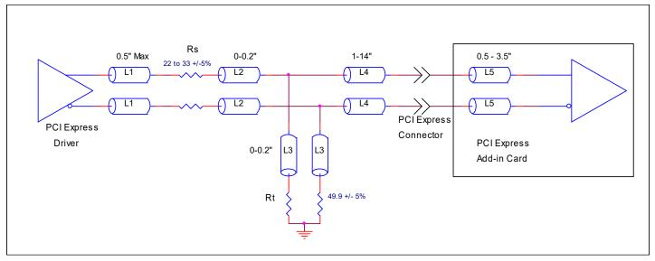
Figure 11A. Recommended Source Termination (where the driver and receiver will be on separate PCBs)
