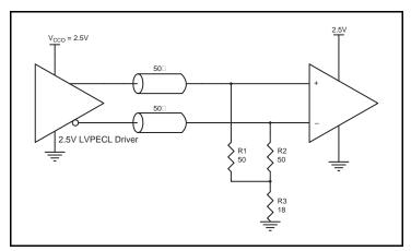
Figure 10C. 2.5V LVPECL Driver Termination Example
