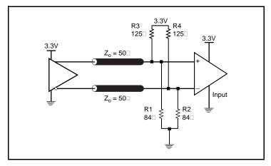
Figure 9B. 3.3V LVPECL Output Termination
