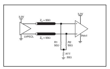
Figure 9A. 3.3V LVPECL Output Termination
