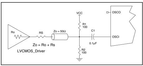
Figure 5A. General Diagram for LVCMOS Driver to XTAL Input Interface
