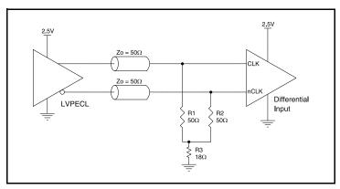
Figure 8C. CLKx/nCLKx Input Driven by a 2.5V LVPECL Driver
