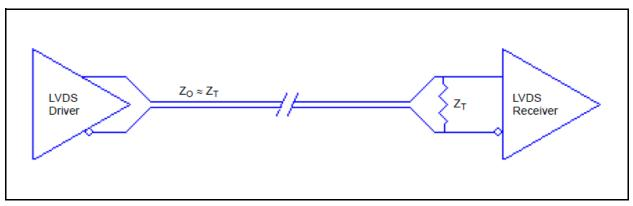
Figure 12A. Standard LVDS Termination
