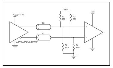
Figure 10A. 2.5V LVPECL Driver Termination Example
