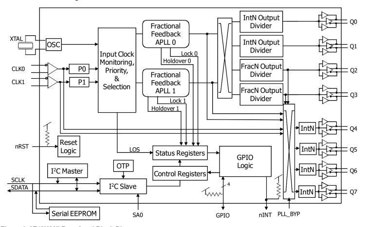
Figure 1. 8T49N287 Functional Block Diagram
