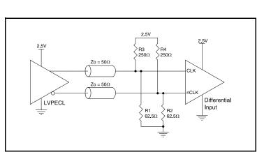
Figure 8B. CLKx/nCLKx Input Driven by a 2.5V LVPECL Driver
