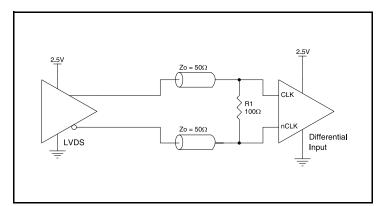
Figure 8D. CLKx/nCLKx Input Driven by a 2.5V LVDS Driver
