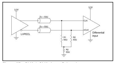
Figure 7D. CLKx/nCLKx Input Driven by a 3.3V LVPECL Driver
