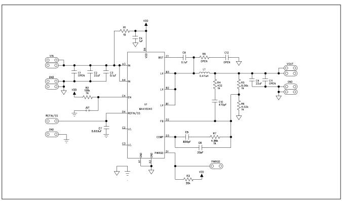
Figure 1. MAX15040 EV Kit Schematic
