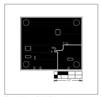
Figure 4. MAX15040 EV Kit PCB Layout—Inner Layer 2
