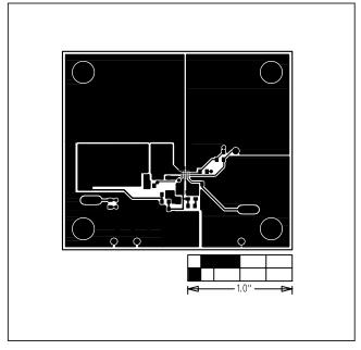
Figure 3. MAX15040 EV Kit Component PCB Layout—Component Side
