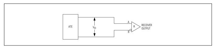
Figure 6. Receiver Propagation Delay Test Circuit
