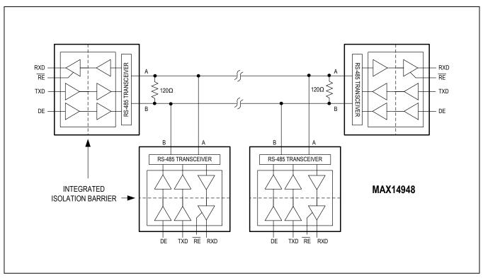
Figure 9. Typical Isolated Half-Duplex RS-485 Application
