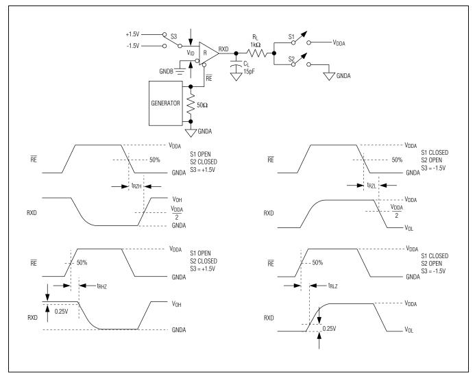
Figure 8. Receiver Enable and Disable Times
