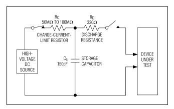
Figure 12. IEC 61000-4-2 ESD Test Model
