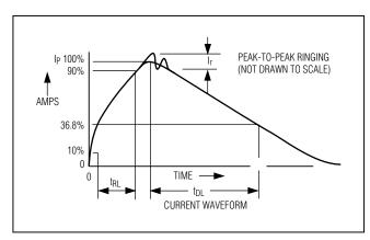
Figure 11. Human Body Current Waveform
