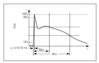
Figure 13. IEC 61000-4-2 ESD Generator Current Waveform
