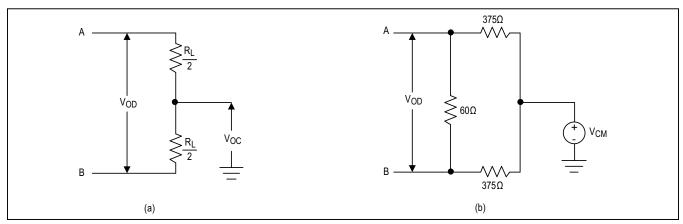
Figure 1. Driver DC Test Load
