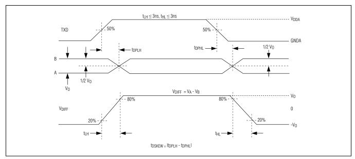
Figure 3. Driver Propagation Delays
