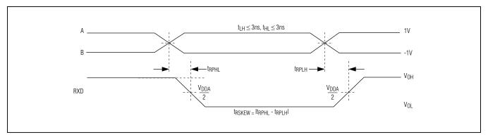
Figure 7. Receiver Propagation Delays
