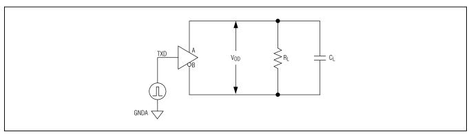
Figure 2. Driver Timing Test Circuit
